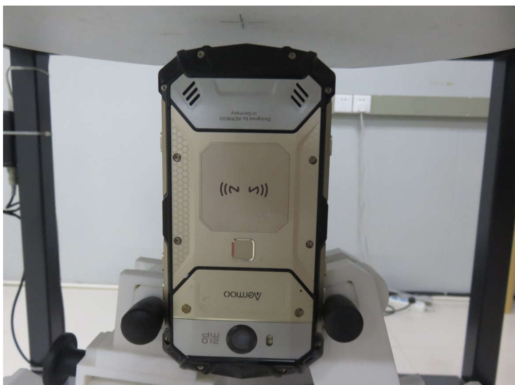
10mm body-worn Bottom Side Setup Photo(hotspot)
