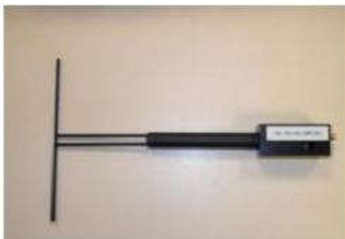
Figure 1 – Satimo COMOSAR Validation Dipole
