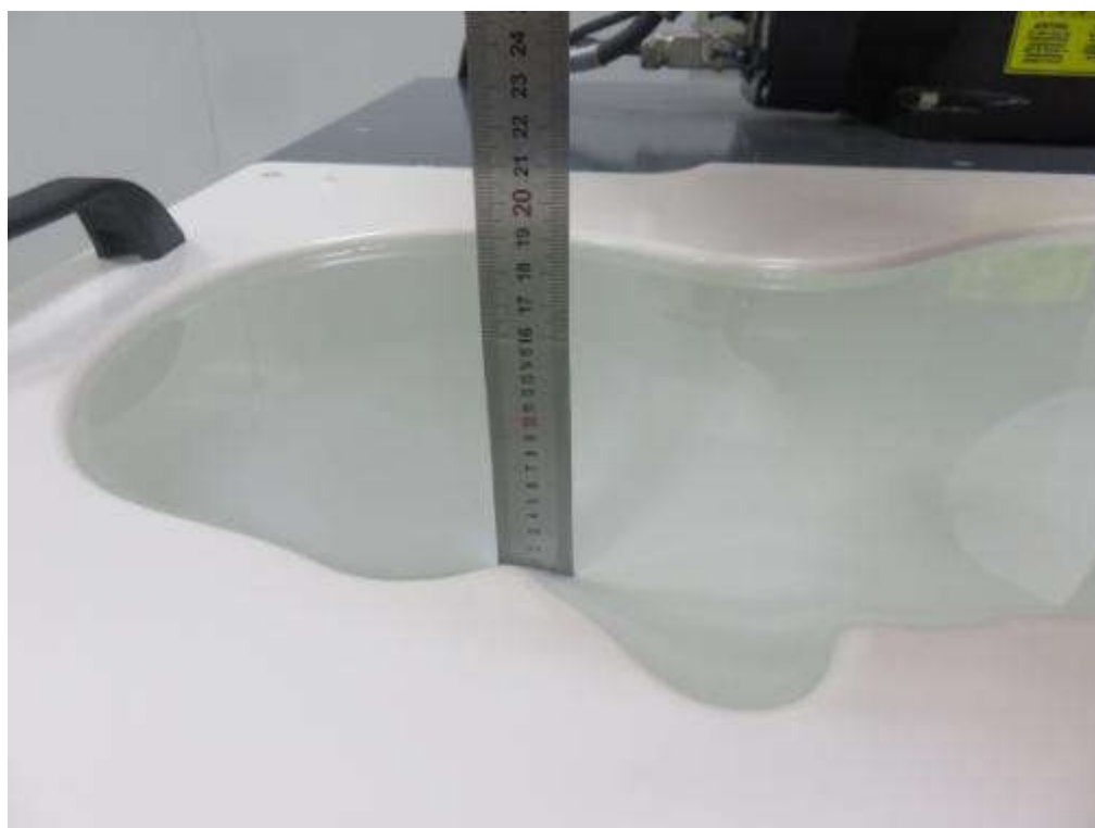
Photograph of the depth in the Head Phantom (1900MHz, 15.7cm depth)
