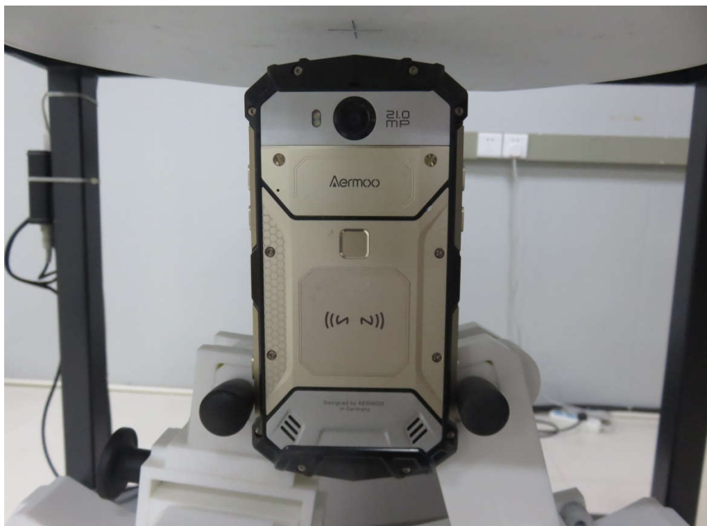
10mm body-worn Top Side Setup Photo(hotspot)
