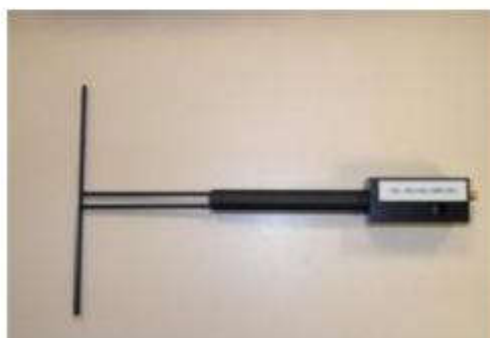
Figure 1 – Satimo COMOSAR Validation Dipole
