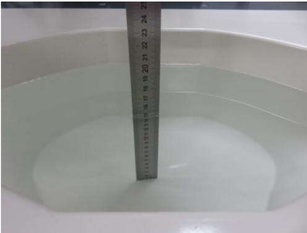
Photograph of the depth in the Body Phantom (2600MHz, 16.2cm depth)
