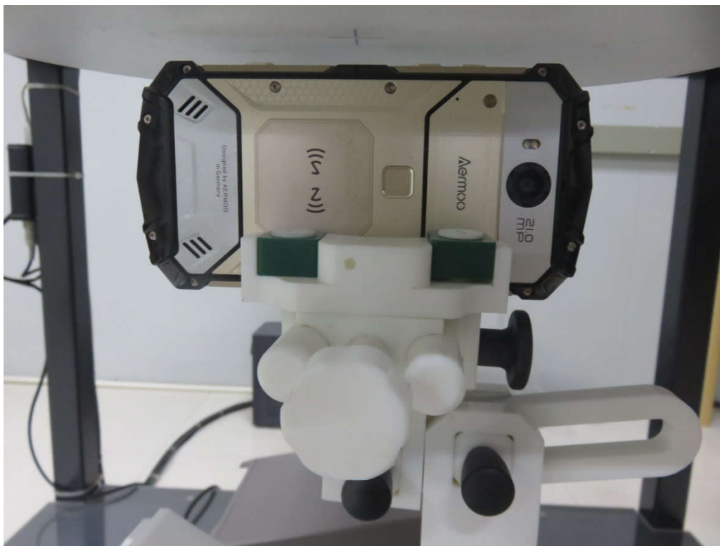
10mm body-worn Right Side Setup Photo(hotspot)
