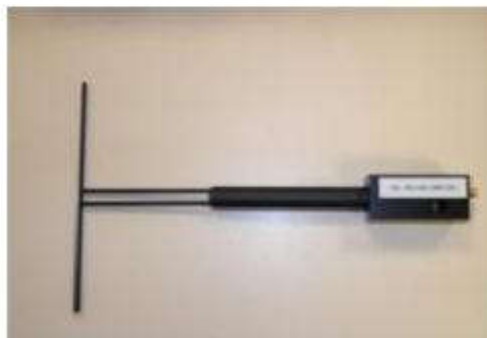
Figure 1 – Satimo COMOSAR Validation Dipole
