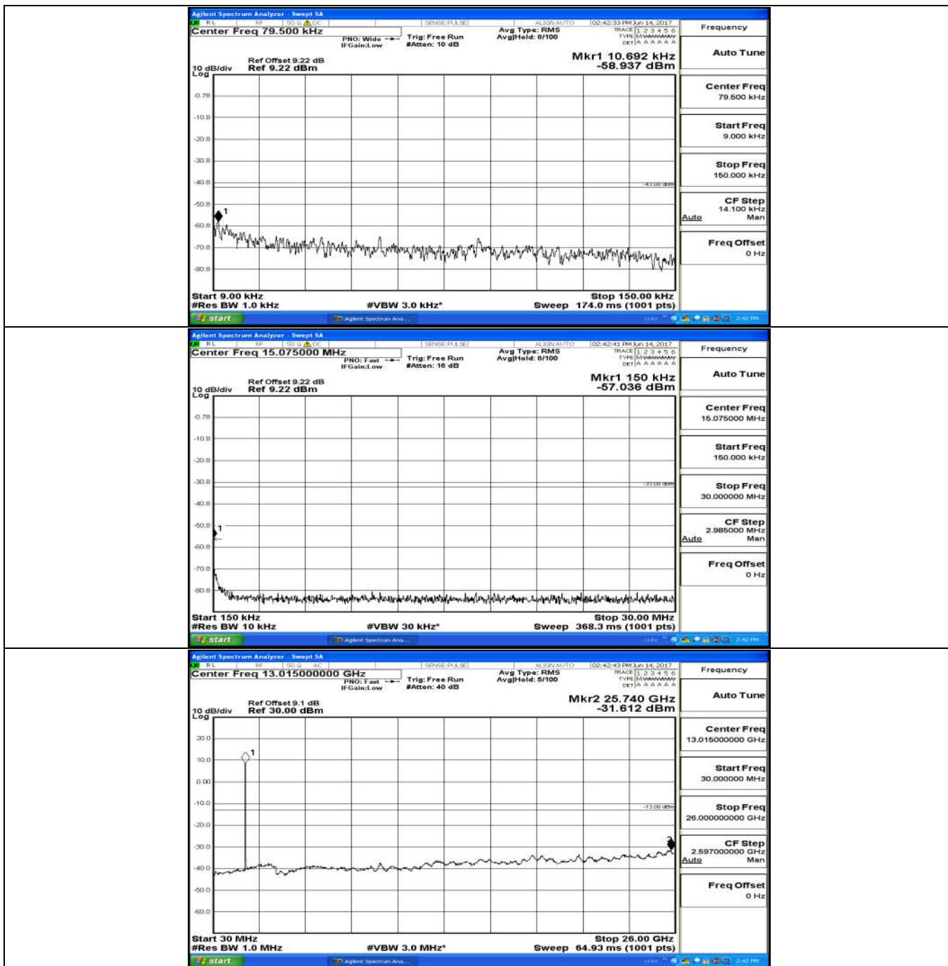
Channel Bandwidth: 10 MHz\_HCH\_16QAM\_50RB#0
