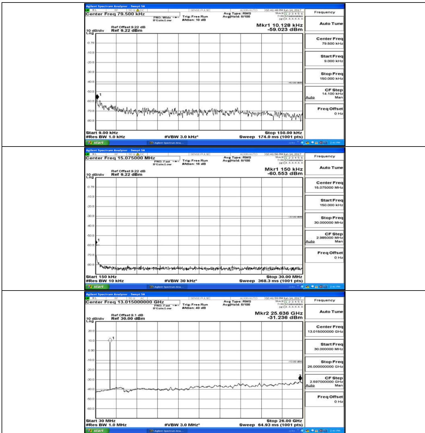
Channel Bandwidth: 10 MHz\_HCH\_QPSK\_50RB#0
