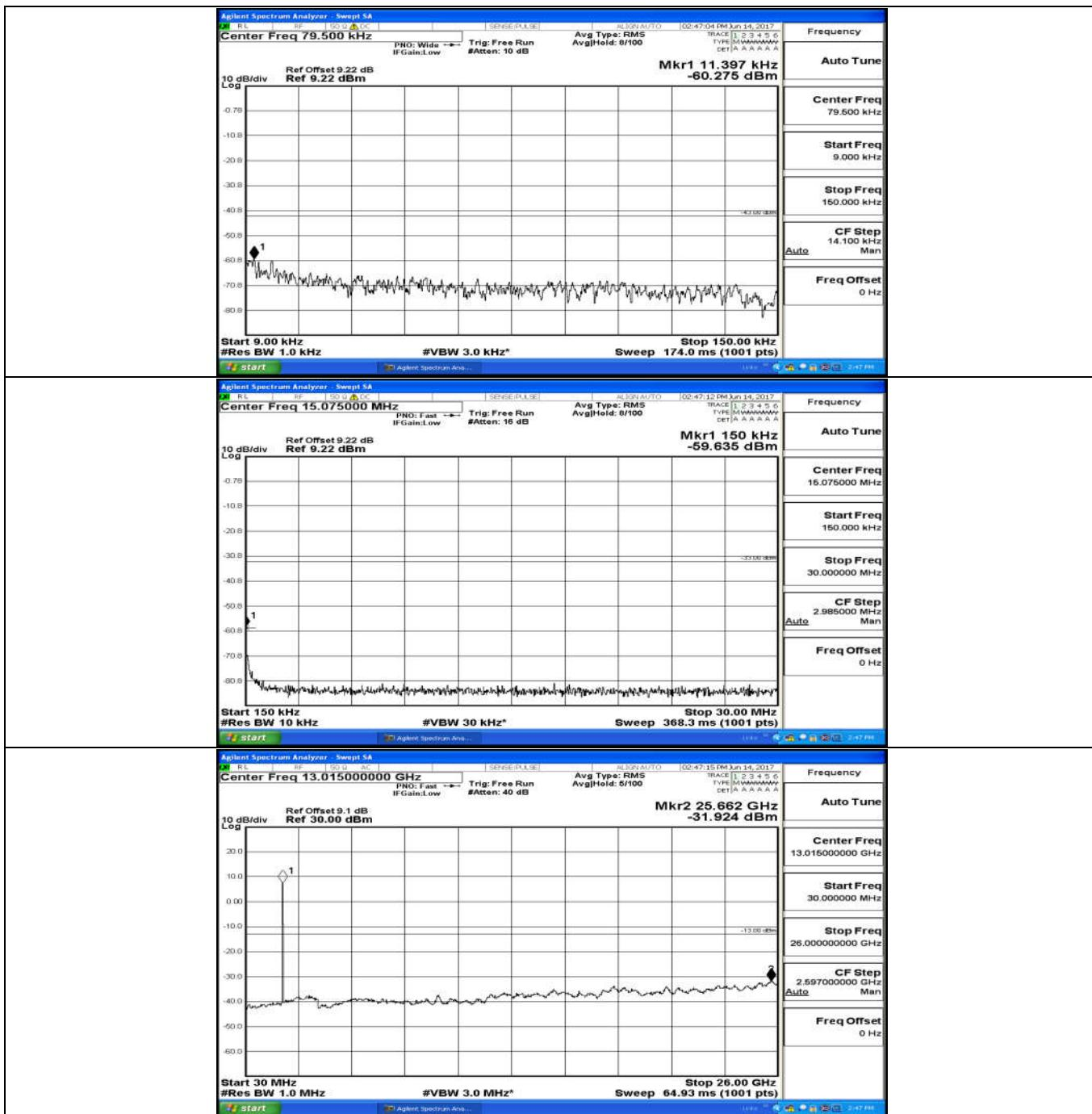
(Channel Bandwidth:15 MHz)\_HCH\_16QAM\_75RB#0
