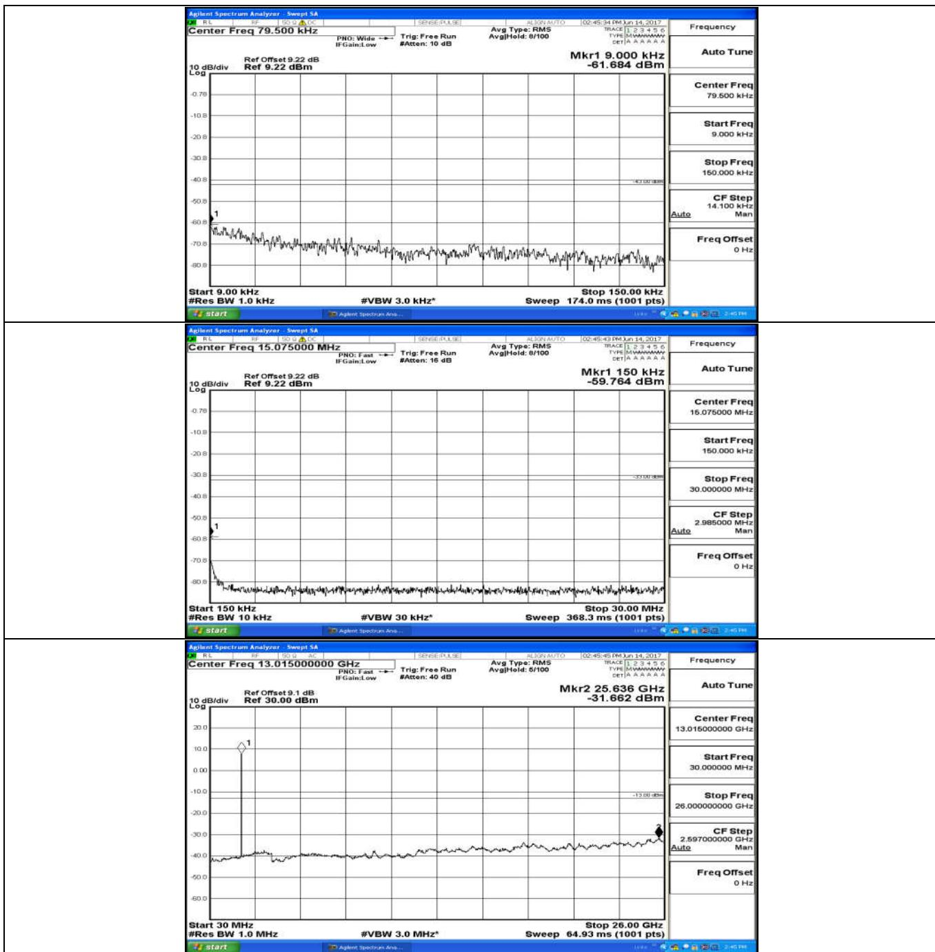
(Channel Bandwidth:15 MHz)\_MCH\_16QAM\_75RB#0
