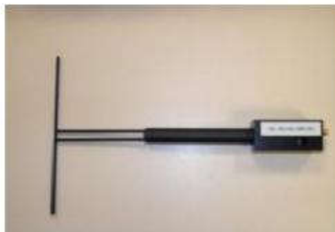
Figure 1 – Satimo COMOSAR Validation Dipole
