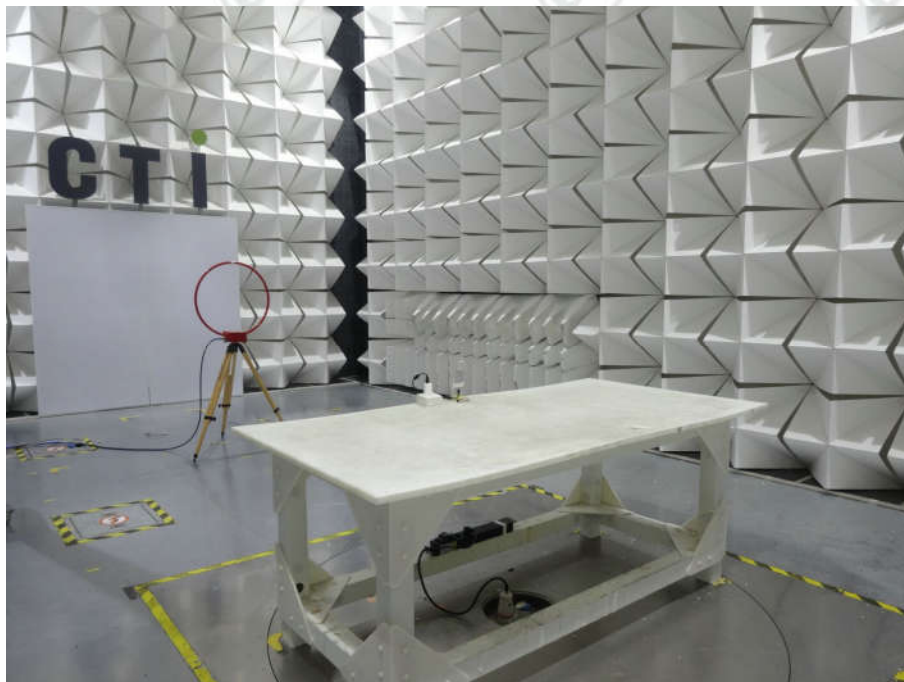
Radiated spurious emission Test Setup-1(Below 30MHz)
