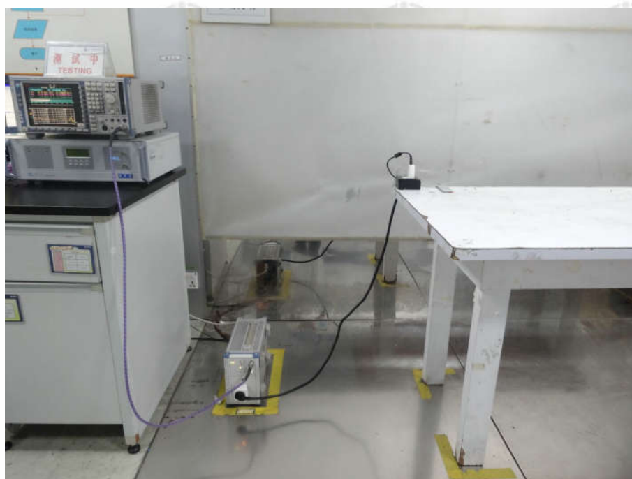
Conducted Emissions Test Setup
