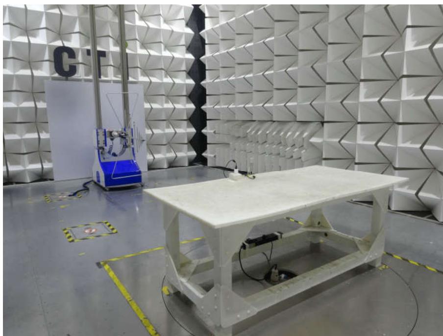
Radiated spurious emission Test Setup-2(30MHz-1GHz)
