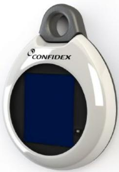
Energy efficient and maintenance free Bluetooth® LE beacon for industrial asset tracking applications and people flow management. Built-in solar panel and power management IC (PMIC) absorbs energy from the surrounding light sources enabling battery free operation and extremely long lifetime. Omnidirectional antenna is designed especially for accurate positioning in both indoor and outdoor applications.
