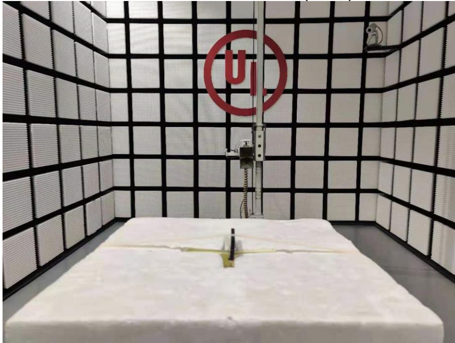
RADIATED RF MEASUREMENT SETUP (30MHz~1GHz)
