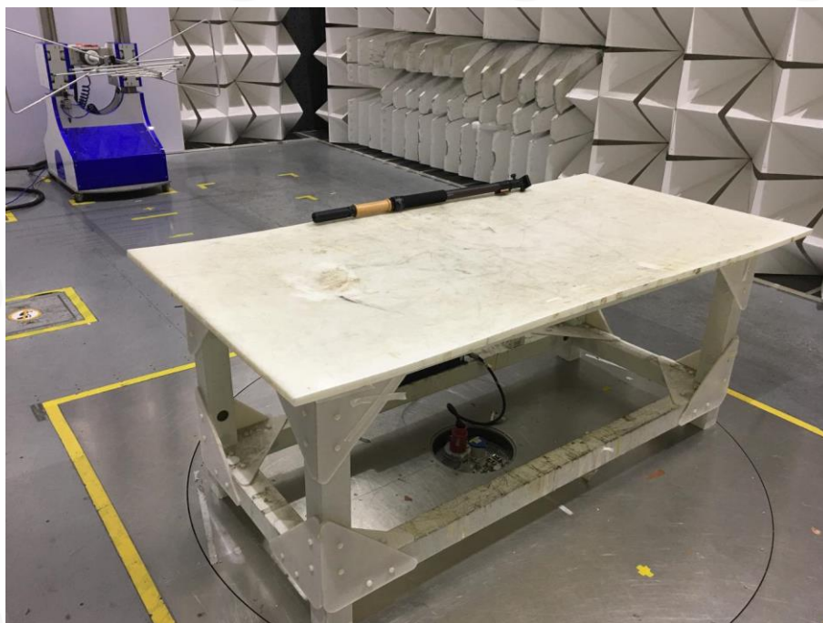
Radiated spurious emission Test Setup-2(Below 1GHz)
