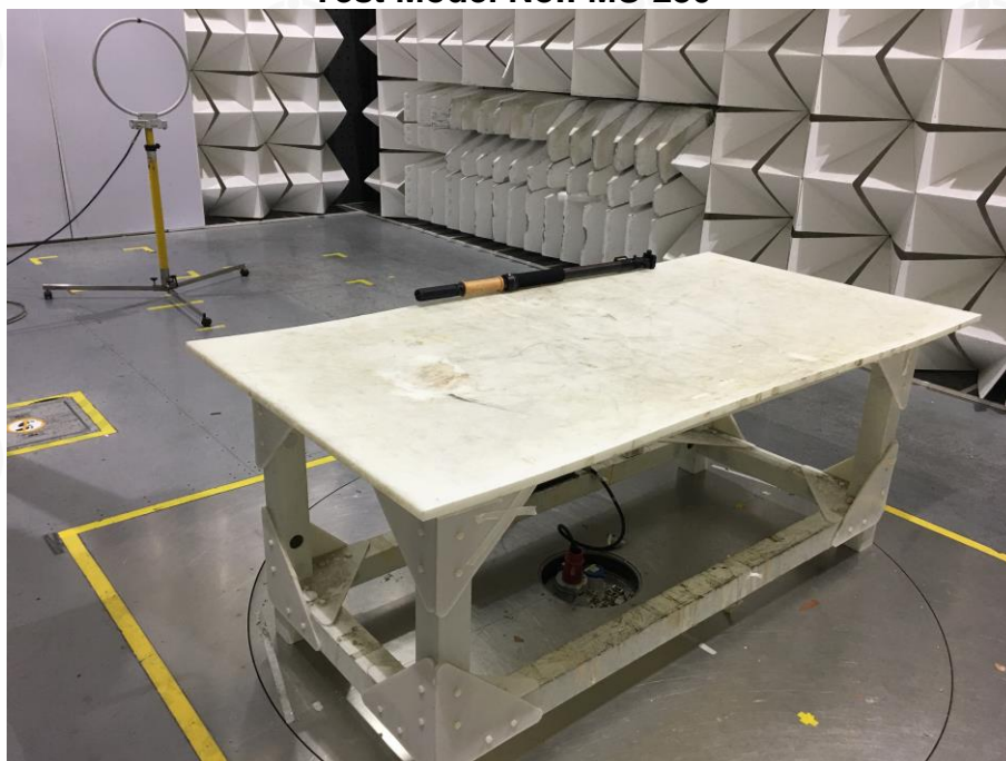
Radiated spurious emission Test Setup-1(Below 30MHz)
