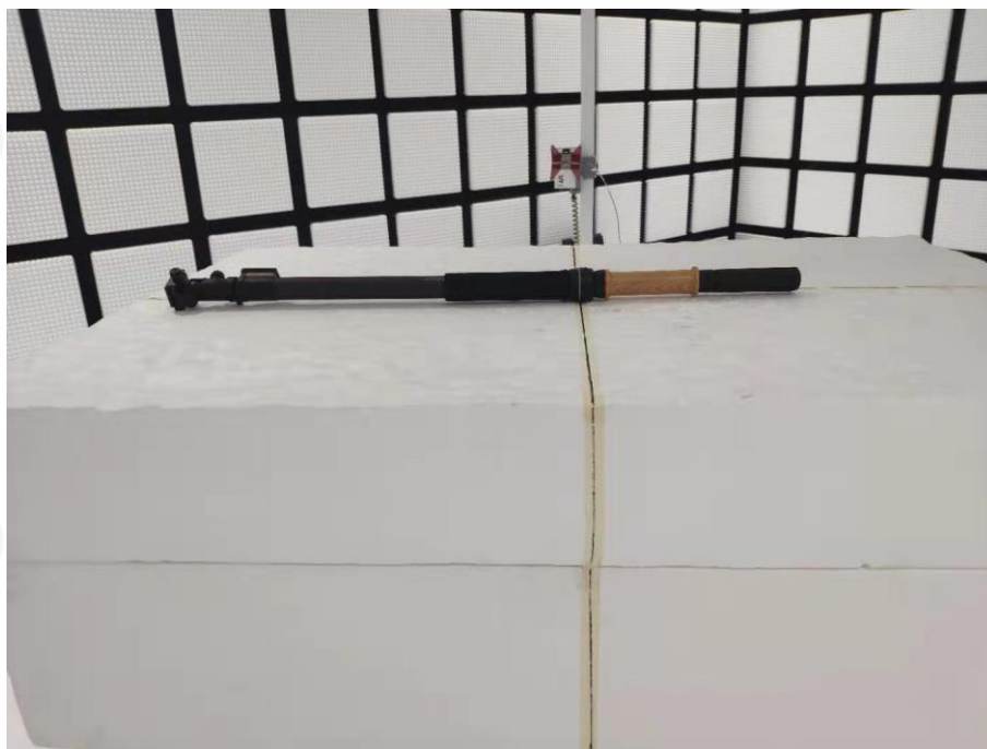
Radiated spurious emission Test Setup-3(Above 1GHz)
