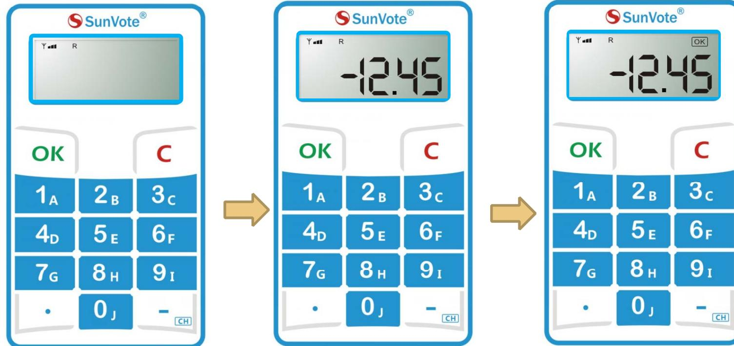
When start **response**, press alphanumeric keys to input your answer and press **【OK】** to submit according to the indication on keypad, and **“OK”** will be displayed after successfully submitting.
