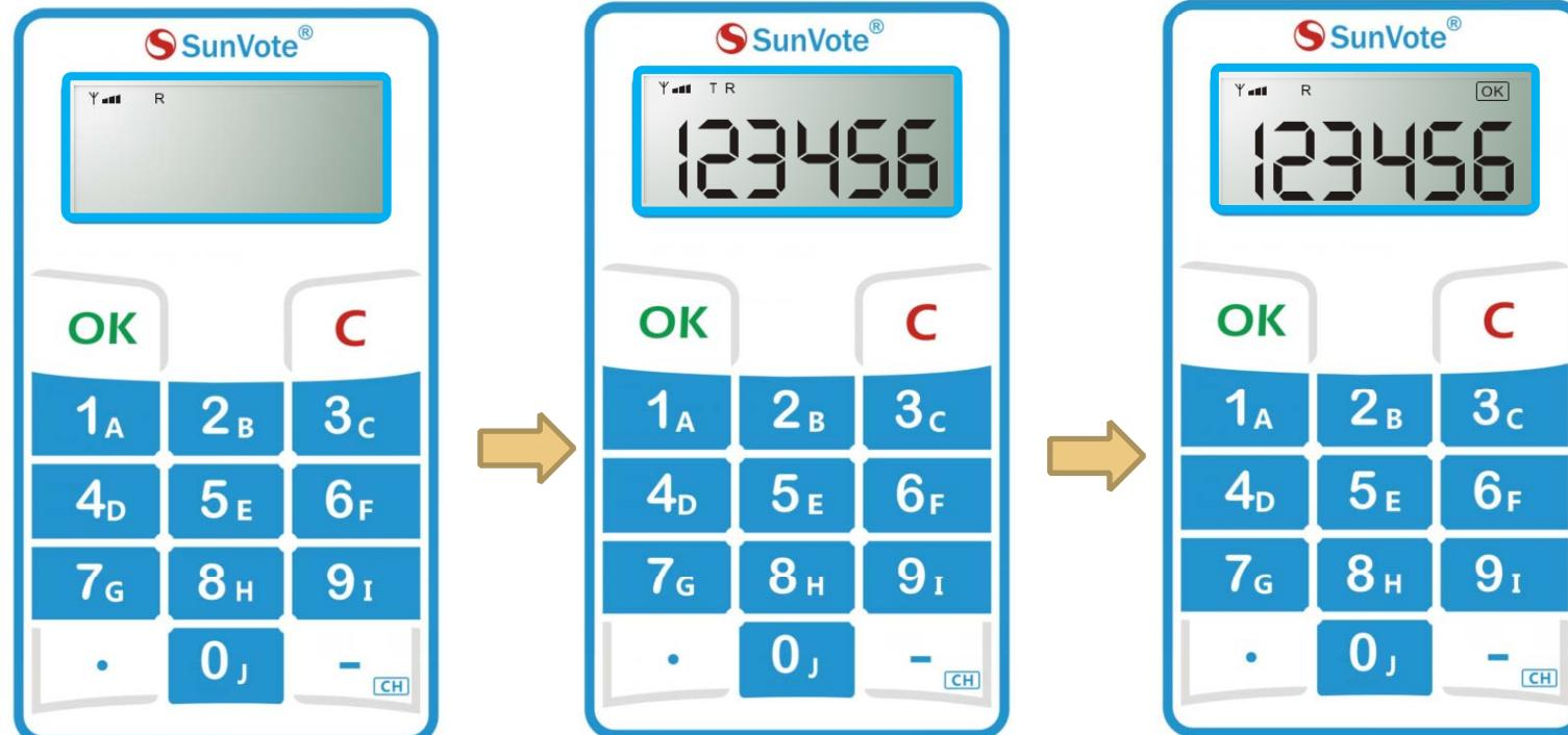
When start **Sign in**, input numbers according to the indication on keypad and press **【OK】** to sign in. "OK" will be displayed after successfully submitting. Max support 16 numeric characters;
