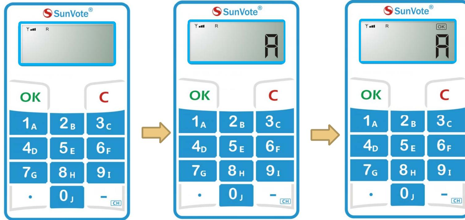
When start **response**, press alphanumeric keys to submit according to the indication on keypad, and “OK” will be displayed after successfully submitting.
