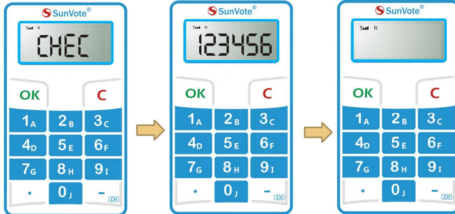
Start **Signin** by software, then input numbers while keypad shows “**CHEC**” and press **【OK】** to sign in. LCD says “OK” after successfully submitting and goes to response interface. If input a wrong code, keypad will say “Err”, and now input a new code. Max support 16 numbers for ID mode and 12 numbers for SN mode;
