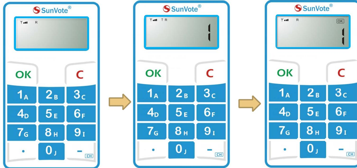
When start **response**, press **【OK】** for fastest response, and “OK” will be displayed after successfully submitting.
