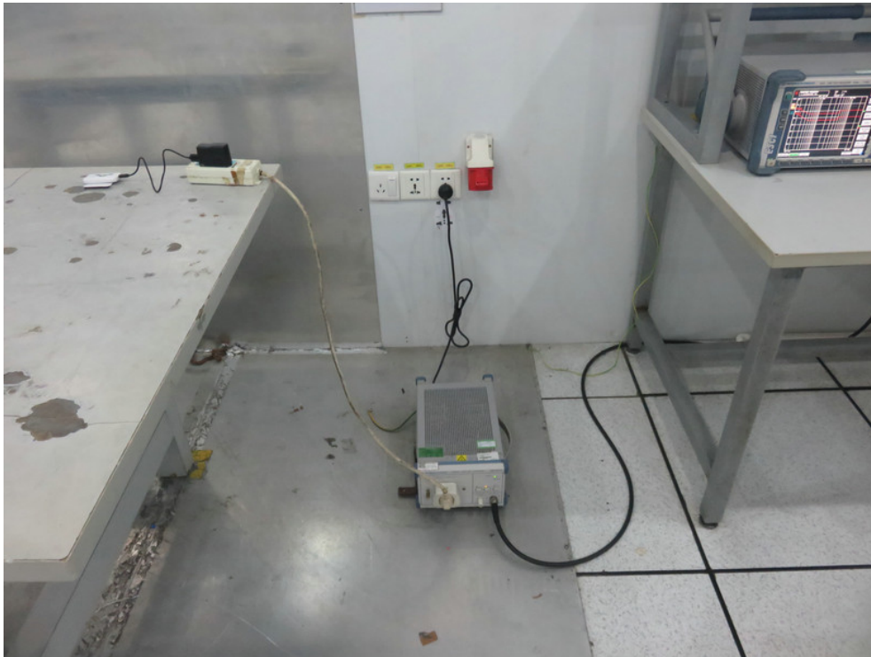
Photo of Conducted Emission Measurement
