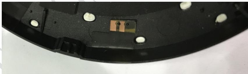
Picture 3 WIFI antenna photograph
