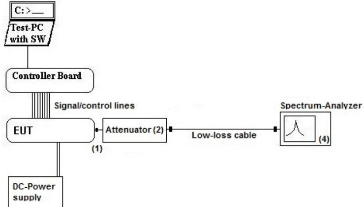
**Testing method:** ANSI C63.10:2013, KDB 558074 D01 DTS Meas.Guidance v03r02
