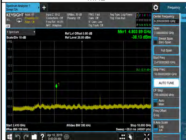
GFSK,2441MHz,DH5,Plot 1,Band Edge
