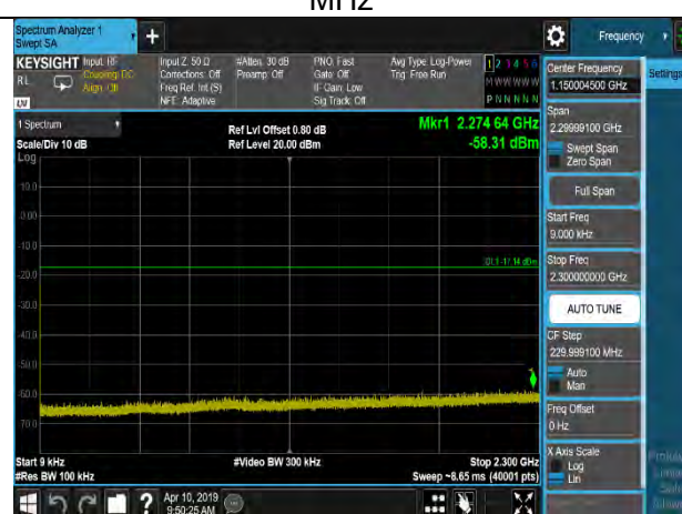
GFSK,2441MHz,DH5,Plot 2,0.009MHz~2300 MHz
