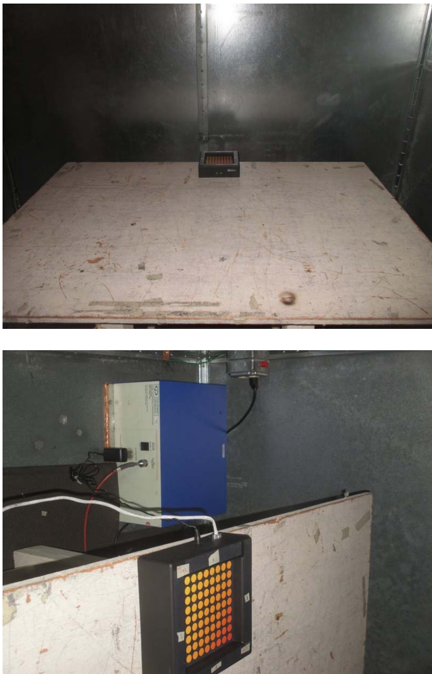
Figure 3.3 Conducted Emission Test Setup
