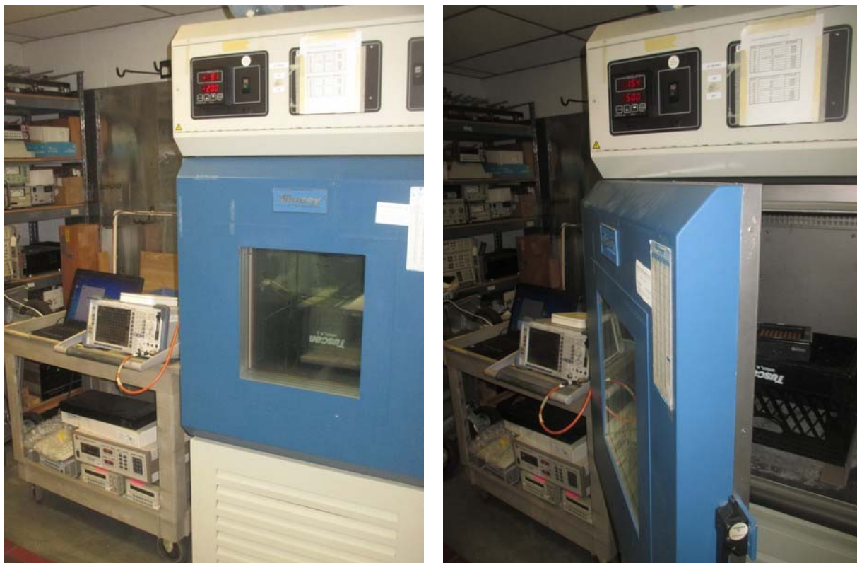
Figure 3.4 Frequency Tolerance Test Setup
