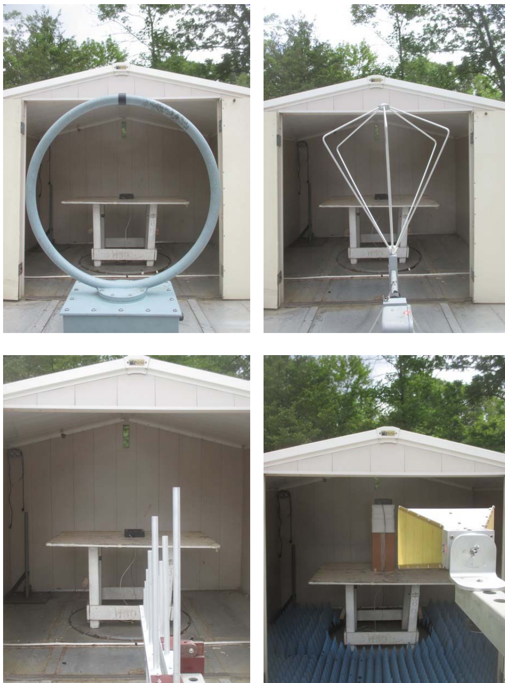
Figure 3.2 Radiated Configuration Test Setup
