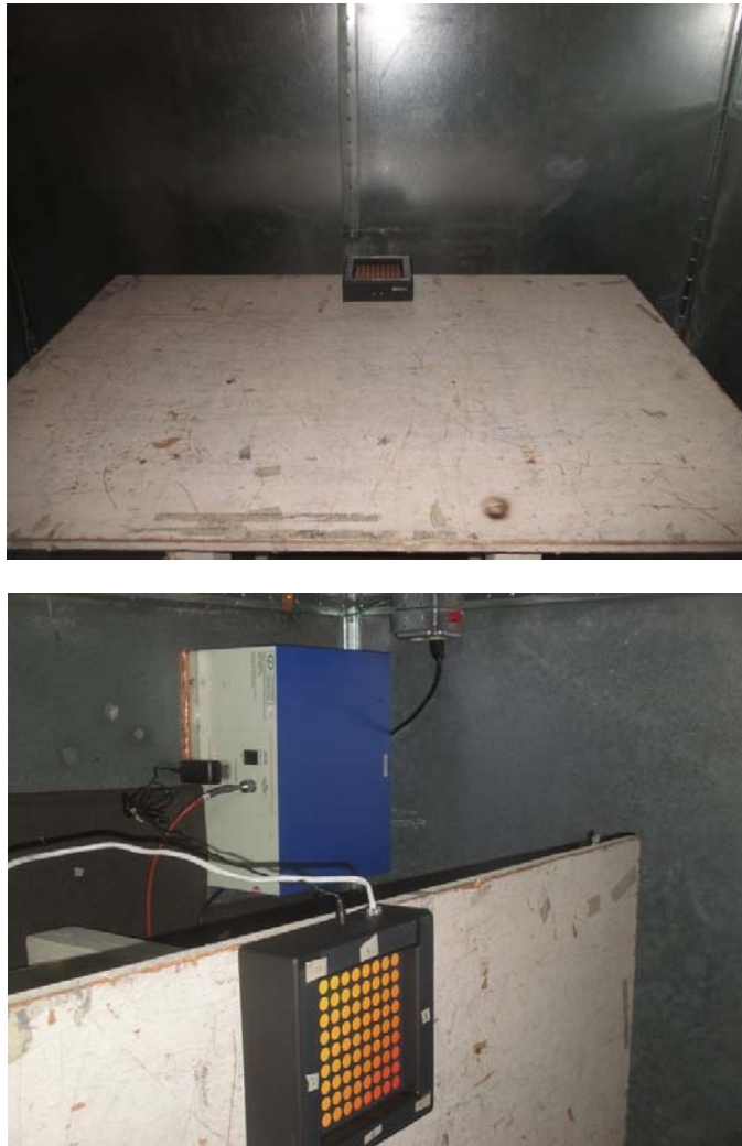
Fig. 3.3 Conducted Emission Test Setup
