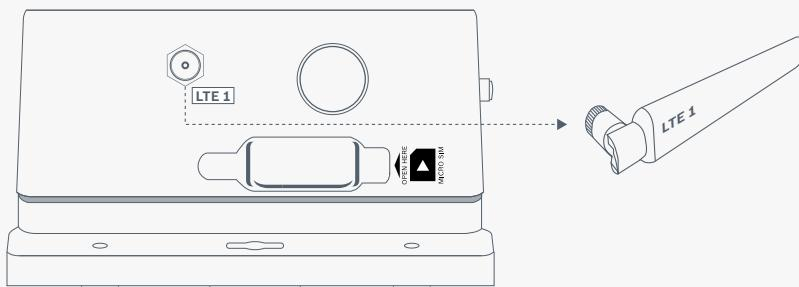
Insert LTE antenna 1 into LTE antenna 1 port and rotate the antenna nut in a clockwise direction until it is firm. Ensure not to overtighten.
