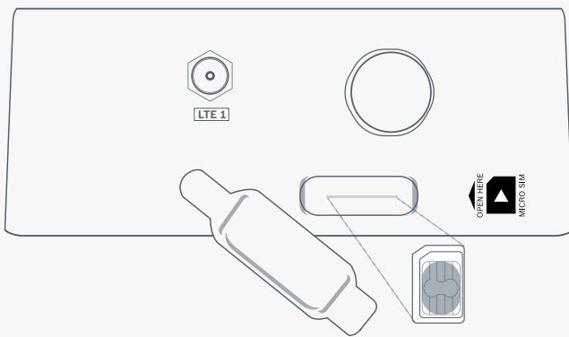
Insert Micro SIM into Phantom Edge as per the marking sticker
