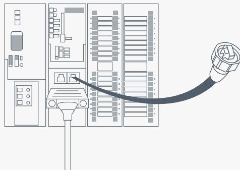
Identify the recommended Amphenol RJ45 Cable RCP-5SAMMM-SLM7Bxx male connector connected to machine PLC
