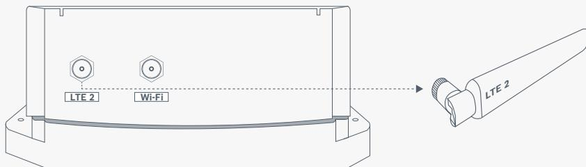
Insert LTE antenna 2 into LTE antenna 2 port and rotate the antenna nut in a clockwise direction until it is firm. Ensure not to overtighten.
