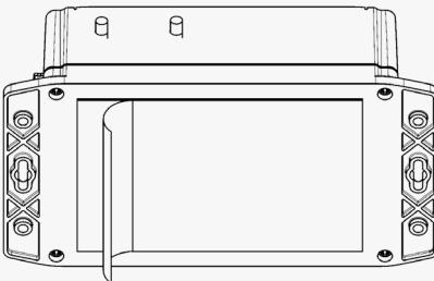
Clean the backside of the device using Iso-Propyl alcohol, peel off the liner from one side of double sided tape and stick it to the backside of Phantom Edge as shown above. Ensure there are no air bubbles while sticking.
