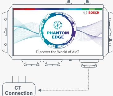
Mount Phantom Edge in a horizontal direction by using adhesive surface of the stickers. Ensure mounting surface is cleaned using Iso-Propyl alcohol before sticking the device.
