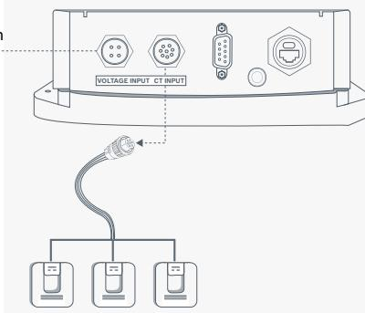
Connect the female connector of this cable to the male connector on Phantom Edge, which is labelled as Voltage Input
