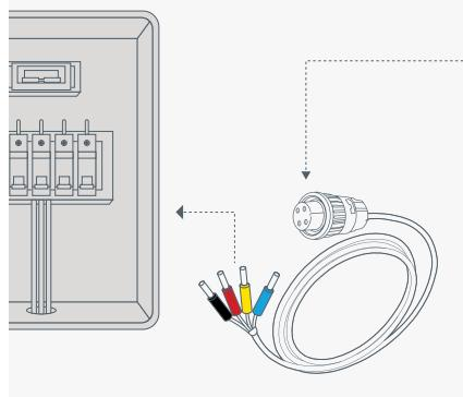
Remove approx. 50mm of insulation from wires. Connect the four-individual wire strands in the voltage connector cable to the appropriate points of the four-pole MCB. Follow color coding of the wire strands to ensure correct connection (Refer exhibit 1).
