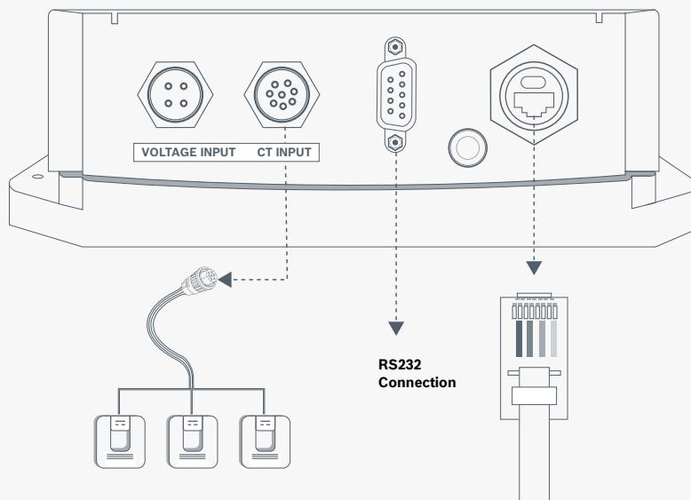
Connect machine's RJ45 ethernet male connector to the RJ45 female port of Phantom Edge and rotate connector nut in a clockwise direction to tighten it
