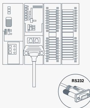
Identify RS232 female connector connected to machine PLC
