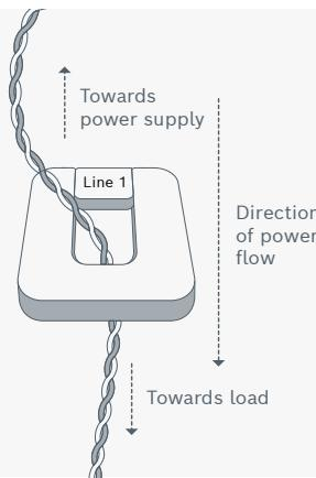
Clamp CT around the individual power cable for each phase. Ensure that the front surface of the CT and line label, is oriented in the direction of power source. Ensure color code of the power cable and line label matches.
