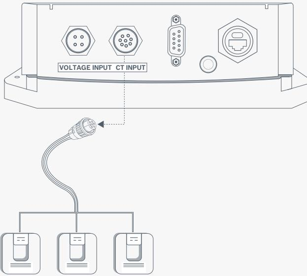
Connect the CT female connector to the male connector on Phantom Edge, which is labelled as Current Input
