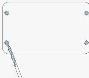
Use the Drill Paper Guide and mark the four locations to drill on the target wall
