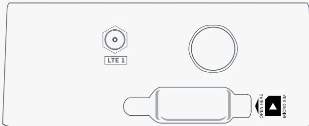
Gently pull the flap on its right side to reveal the Micro SIM card slot
