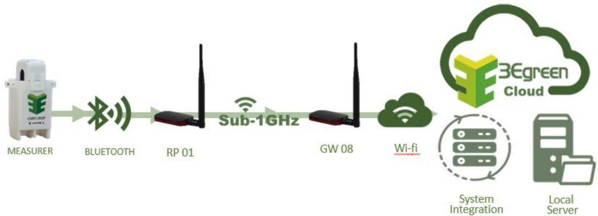
RP01 receives the data from the measurer then passes through the data into GW08 which is a sub-1G to WIFI gateway .
