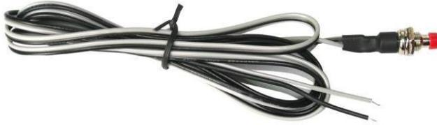
The SOS function need installing the external SOS button, install the external SOS button in a hidden place that driver can press the button, connect one wire of the SOS button to GND (car body), another wire of the SOS button to the tracker SOS wire is OK.
