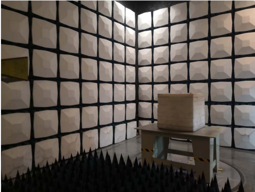
Radiated Emission Above 1GHz View
