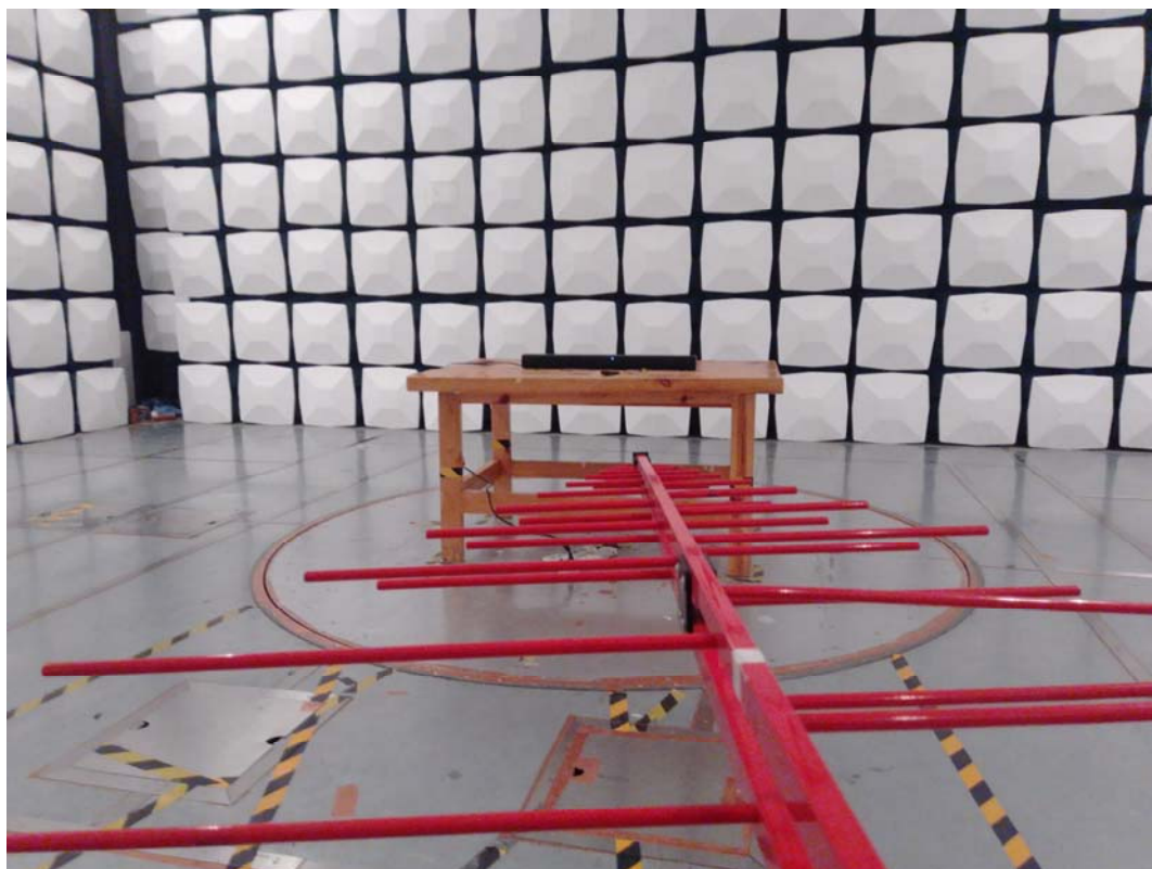
Radiated Emission Above 1GHz View
