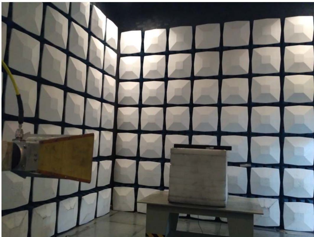
Radiated Emission Above 1GHz View
