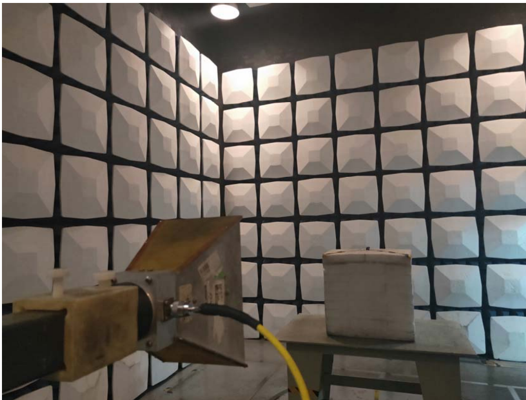
Radiated Emission Above 1GHz View
