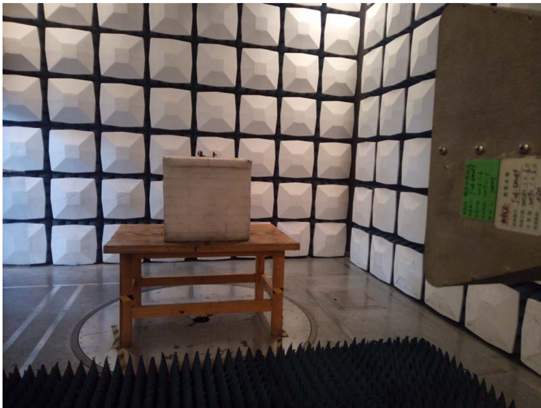
Radiated Emission Above 1GHz View
