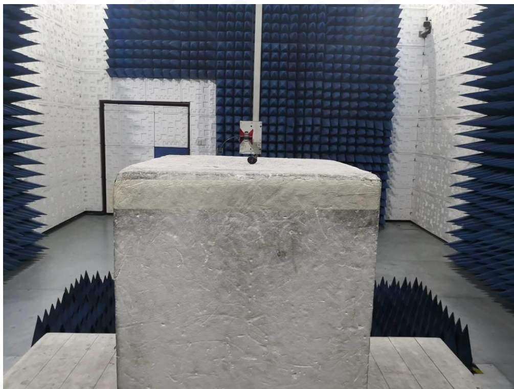
RADIATED EMISSION TEST SETUP ABOVE 1GHZ
