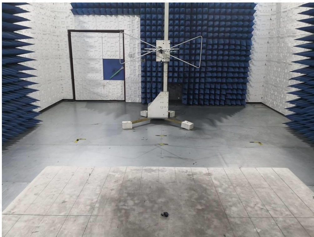
RADIATED EMISSION TEST SETUP ABOVE 1GHZ
