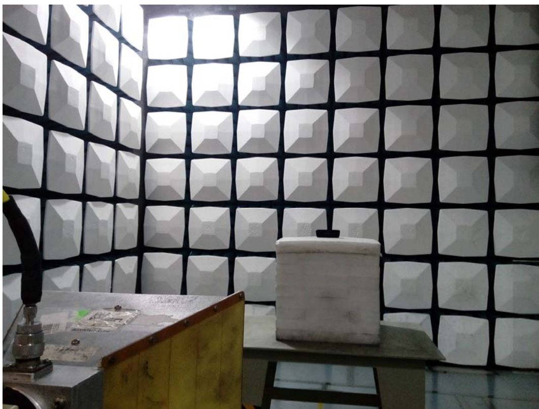
Radiated Emission Above 1GHz View
