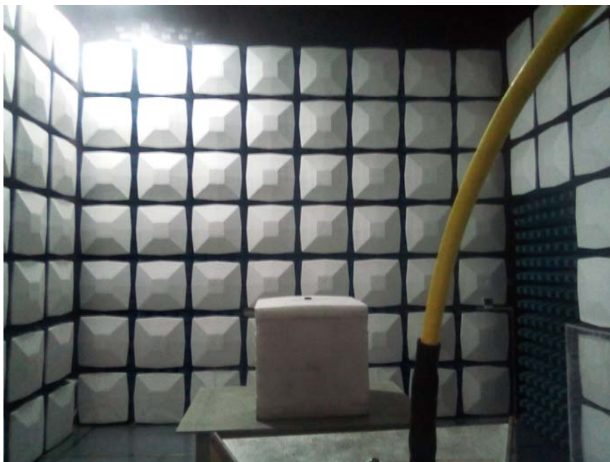
Radiated Emission View (Above 1GHz)
