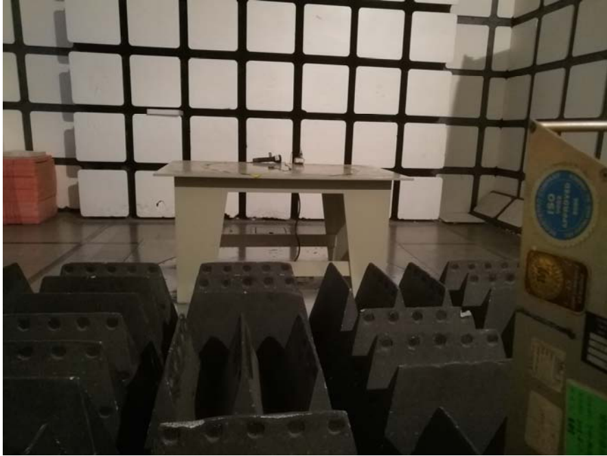
Radiated Emissions – Front View (Above 1 GHz)
