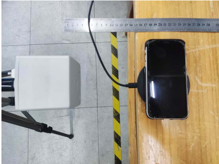
Test Position C-15cm from the edge of EUT to the geometric center of the probe
