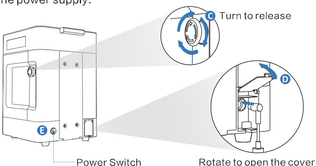
**E** Press the power switch to turn it on. The outer lid opens, and the platform mount and basket raise in position.
