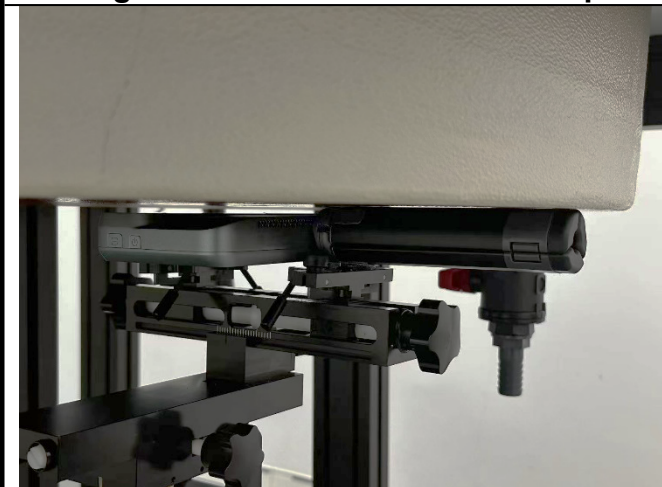
Rear Face of EUT with 0.5 cm Gap + Support
