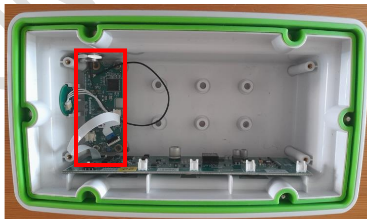
Figure 7 Internal view of F3N1-DIN showing F3N_NF PCB connected to the Digital Node Interface board within the FlatMesh Digital Interface Node (F3N1-DIN)
