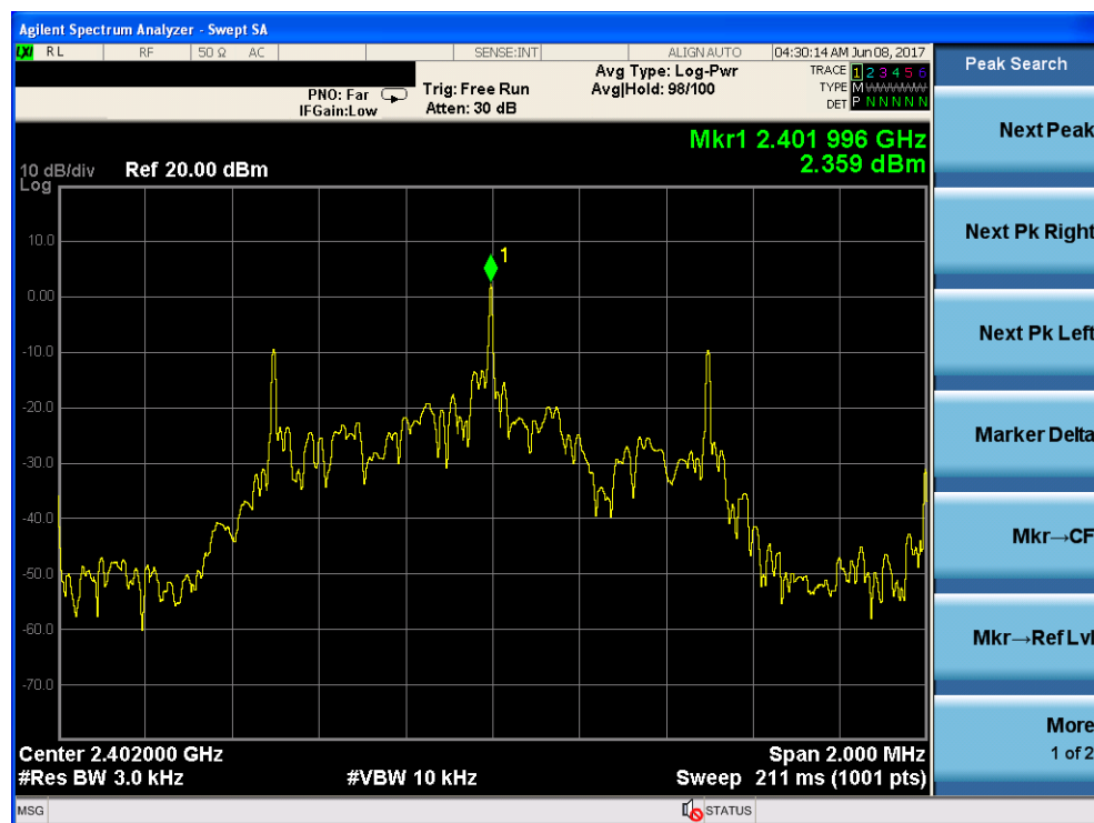
Power spectral density plot on channel 00
