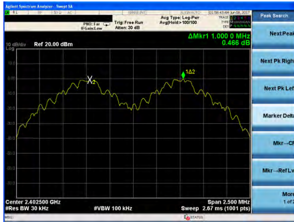
(1Mbps) Channel Separation plot on channel 39-40
