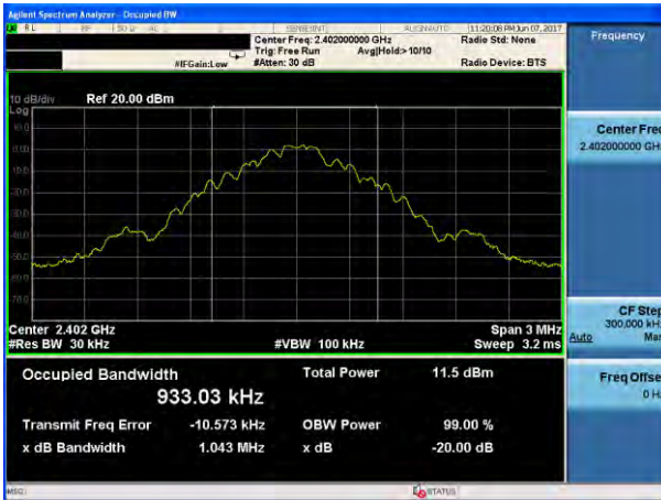
20dB Bandwidth plot on channel 39 (1Mbps)
