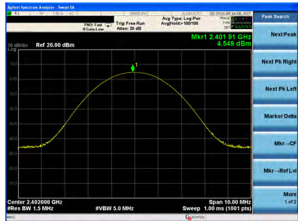
Peak output Power plot on channel 39 (2Mbps)
