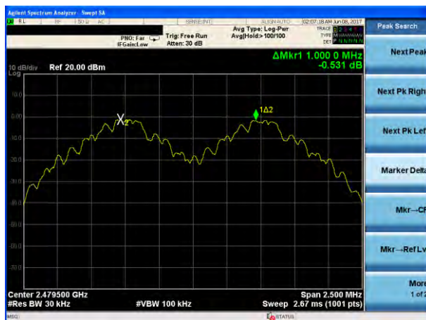
(1Mbps) Channel Separation plot on channel 77-78
