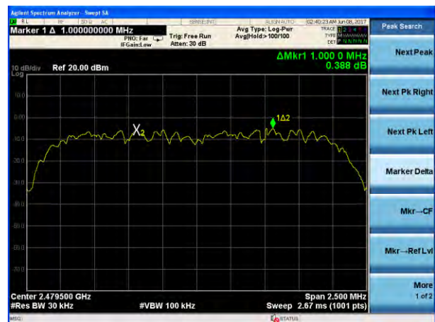
(2Mbps) Channel Separation plot on channel 77-78
