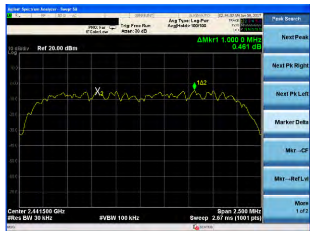
(2Mbps) Channel Separation plot on channel 39-40
