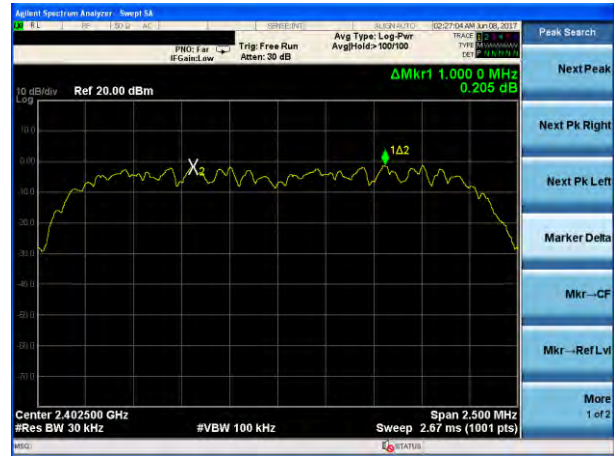
(2Mbps) Channel Separation plot on channel 39-40
