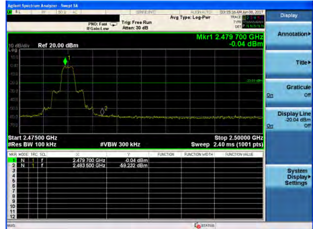
\pi /4-DQPSK: Band Edge-High Channel (Hopping Mode)
