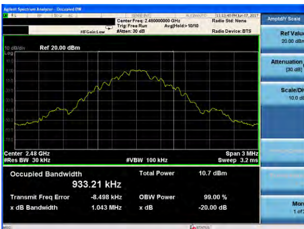
20dB Bandwidth plot on channel 78 (1Mbps)
