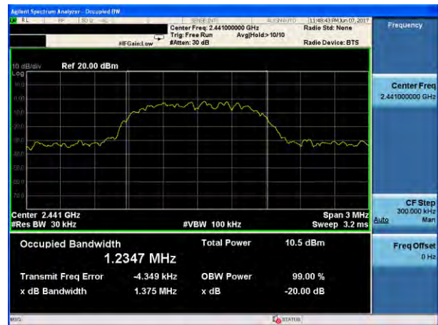
20dB Bandwidth plot on channel 39 (2Mbps)
