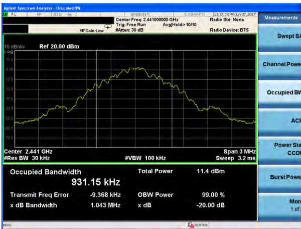
20dB Bandwidth plot on channel 39 (1Mbps)
