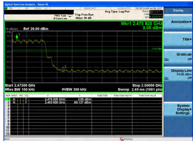
8DPSK: Band Edge-High Channel (Hopping Mode)
