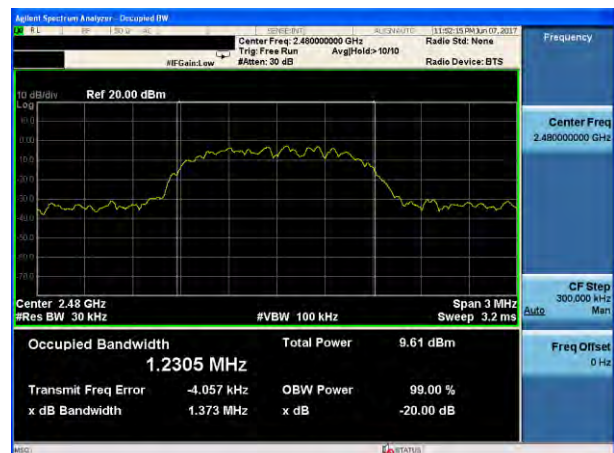
20dB Bandwidth plot on channel 78 (2Mbps)
