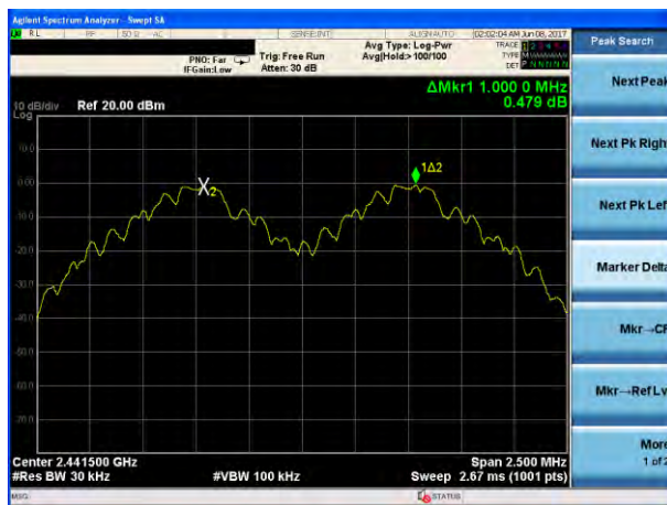
(1Mbps) Channel Separation plot on channel 39-40
