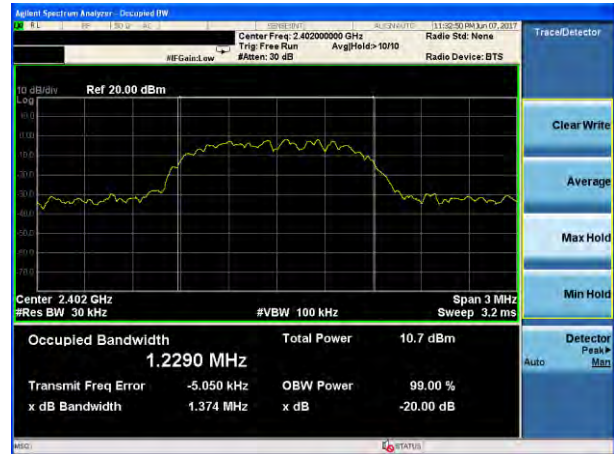
20dB Bandwidth plot on channel 39 (2Mbps)
