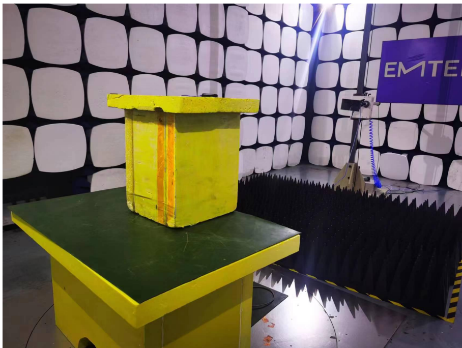
Spurious Emission Test Setup (Above 1GHz)
