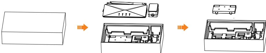
Figure 4-1 Unpacking the ECC-B
