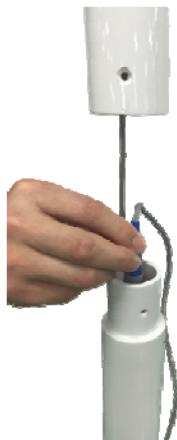
③ As the cable connector is exposed from the other end of the vertical pole, align the notch at the bottom end of the vertical pole with the horizontal pole as shown:
