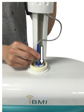
⑥ The connector must be aligned and inserted completely as shown in the arrow-indicated direction and the remaining cable needs to be secured inside the notch.
