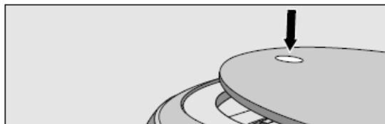
2. Unlatch the dust box by lifting the handle upward
