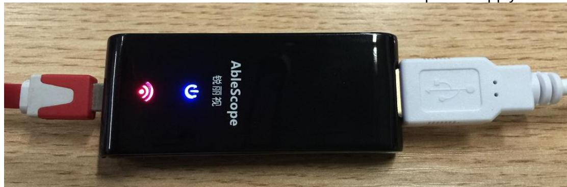
1-1, Plug the camera into the USB port of the WiFi converter
