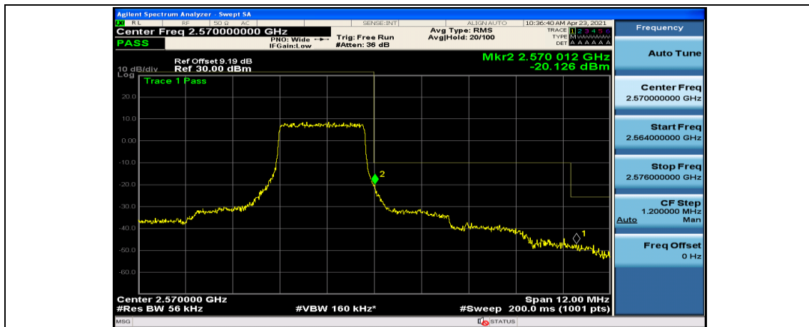
(Channel Bandwidth: 5 MHz)_HCH_QPSK_25RB#0
