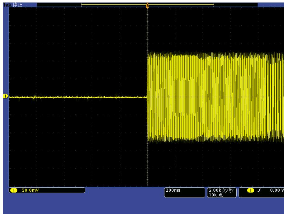
Transmitter Frequency Behaviour @ 25.0 KHz Channel Separation-----On – Off
