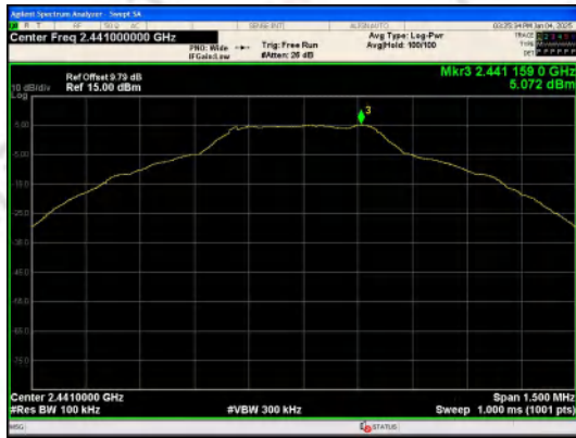
In-Band Reference Level GFSK_DH5_Channel 39
