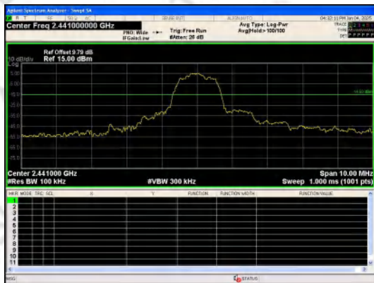
Out Of Band Emission 8DPSK_3-DH1_Channel 39
