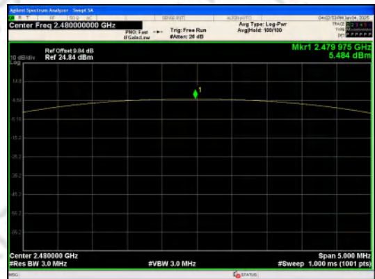
Peak Output Power GFSK_Channel 78
