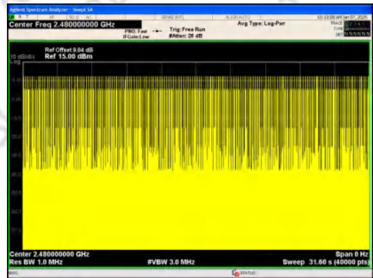
Number of Pulses in 31.6 seconds 8DPSK_3-DH1
