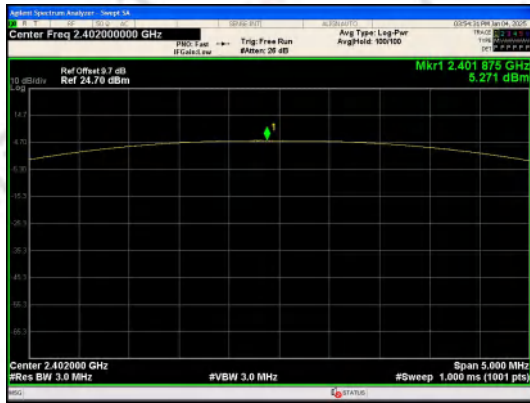
Peak Output Power GFSK_Channel 0
