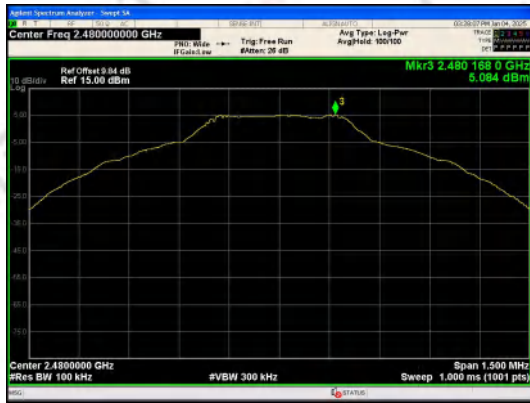
In-Band Reference Level GFSK_DH5_Channel 78
