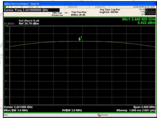
Peak Output Power GFSK_Channel 39
