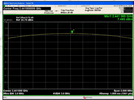
Peak Output Power \pi/4 DQPSK_Channel 39
