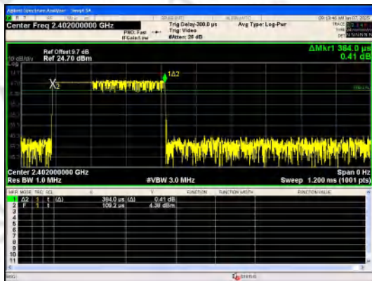
Pulse Width \pi/4 DQPSK_2-DH1
