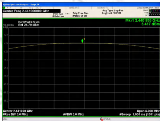
Peak Output Power GFSK_Channel 39
