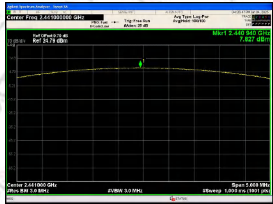
Peak Output Power 8DPSK_Channel 39
