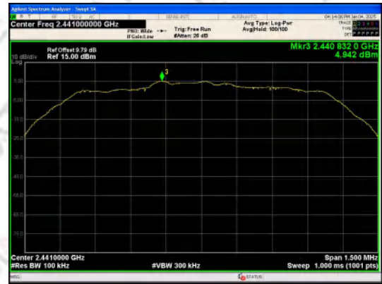
In-Band Reference Level \pi/4 DQPSK_2-DH1_Channel 39
