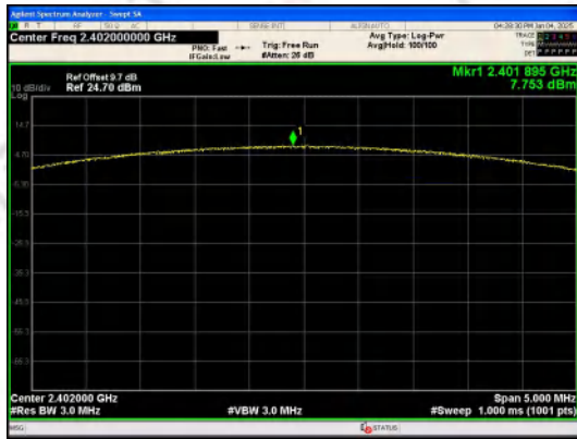
Peak Output Power 8DPSK_Channel 0
