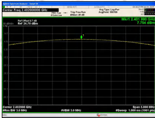
Peak Output Power 8DPSK_Channel 0
