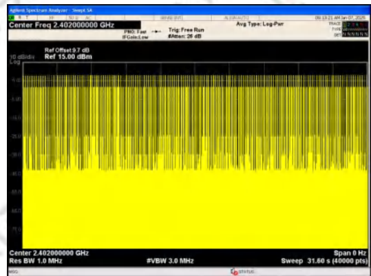
Number of Pulses in 31.6 seconds \pi/4 DQPSK_2-DH1
