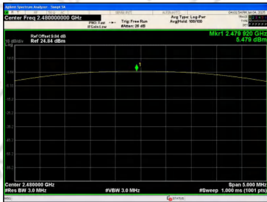
Peak Output Power GFSK_Channel 78
