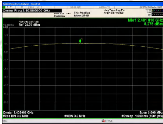
Peak Output Power GFSK_Channel 0
