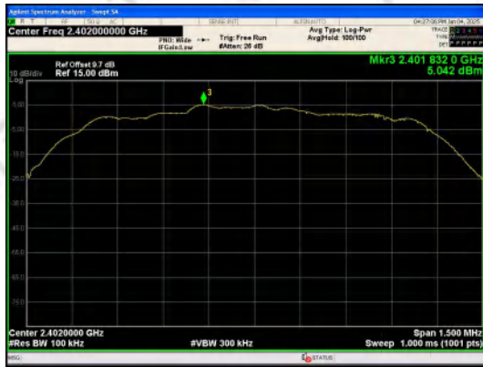
In-Band Reference Level 8DPSK_3-DH1_Channel 0
