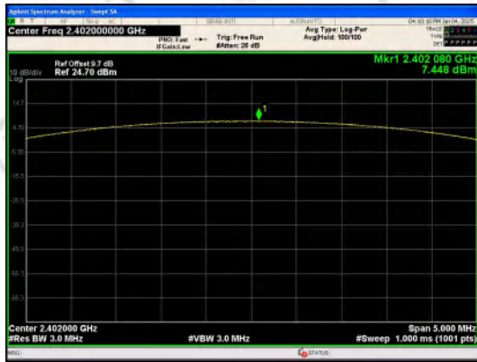
Peak Output Power \pi/4 DQPSK_Channel 0
