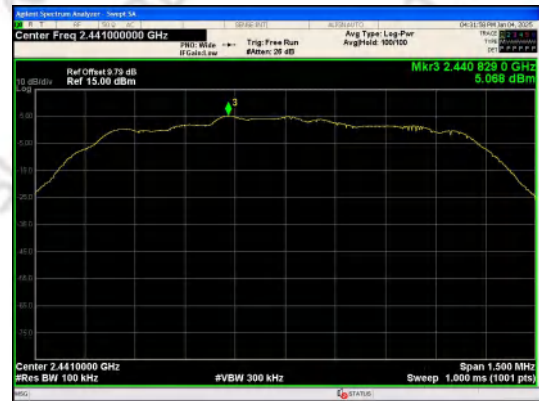
In-Band Reference Level 8DPSK_3-DH1_Channel 39
