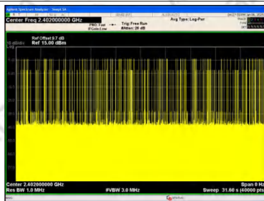
Number of Pulses in 31.6 seconds GFSK_DH5
