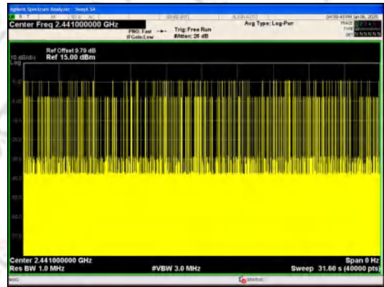
Number of Pulses in 31.6 seconds GFSK_DH5
