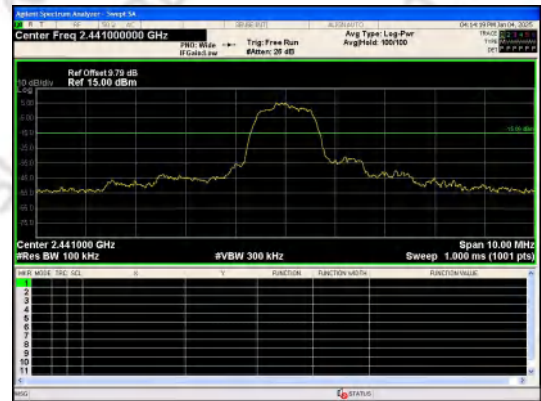
Out Of Band Emission \pi/4 DQPSK_2-DH1_Channel 39
