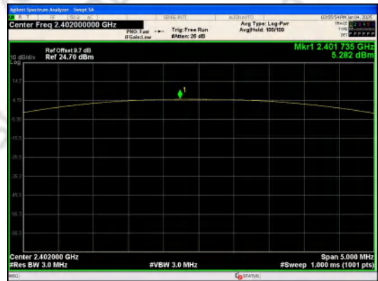
Peak Output Power GFSK_Channel 0
