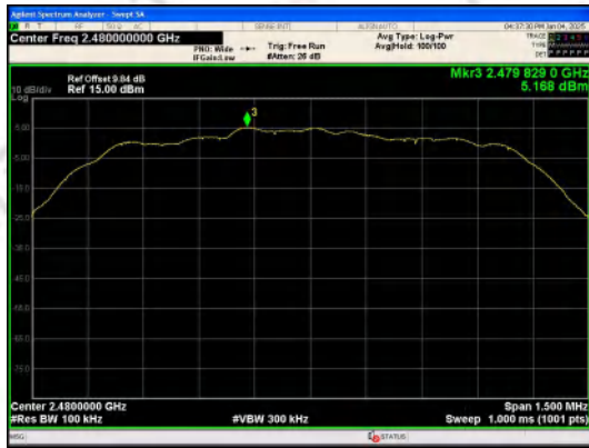
In-Band Reference Level 8DPSK_3-DH1_Channel 78
