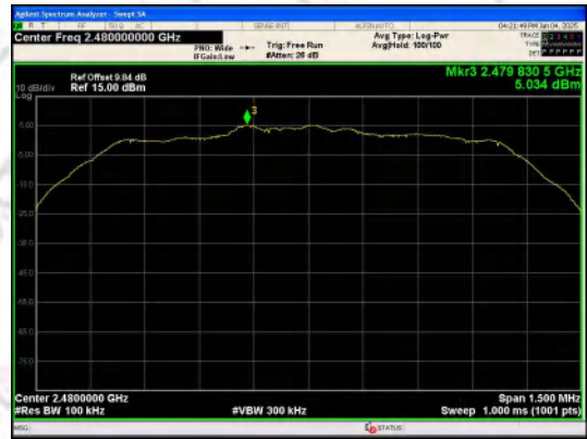
In-Band Reference Level \pi/4 DQPSK_2-DH1_Channel 78
