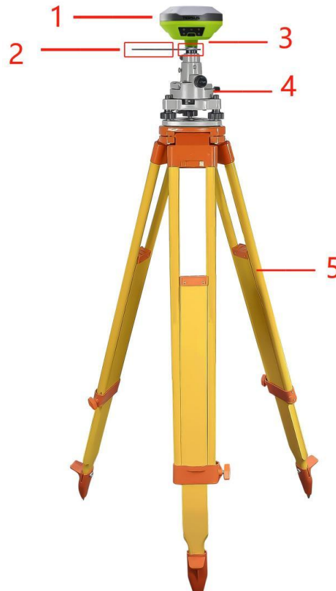
Figure 2.2 LUKA as a base without radio antenna
