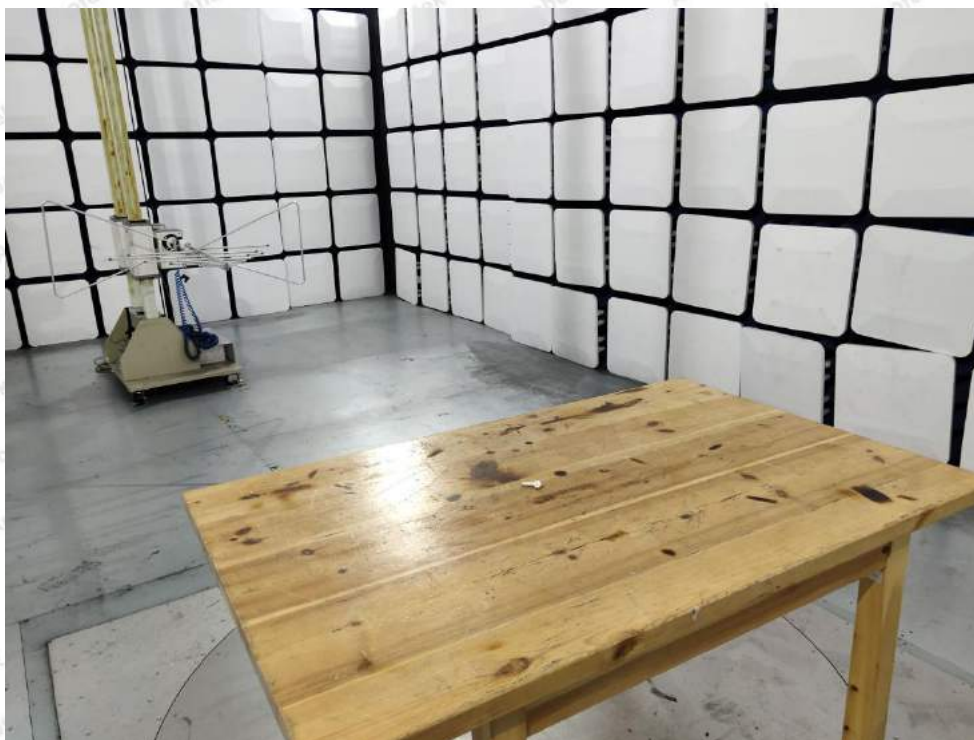
Photo of Radiation Emission Test
