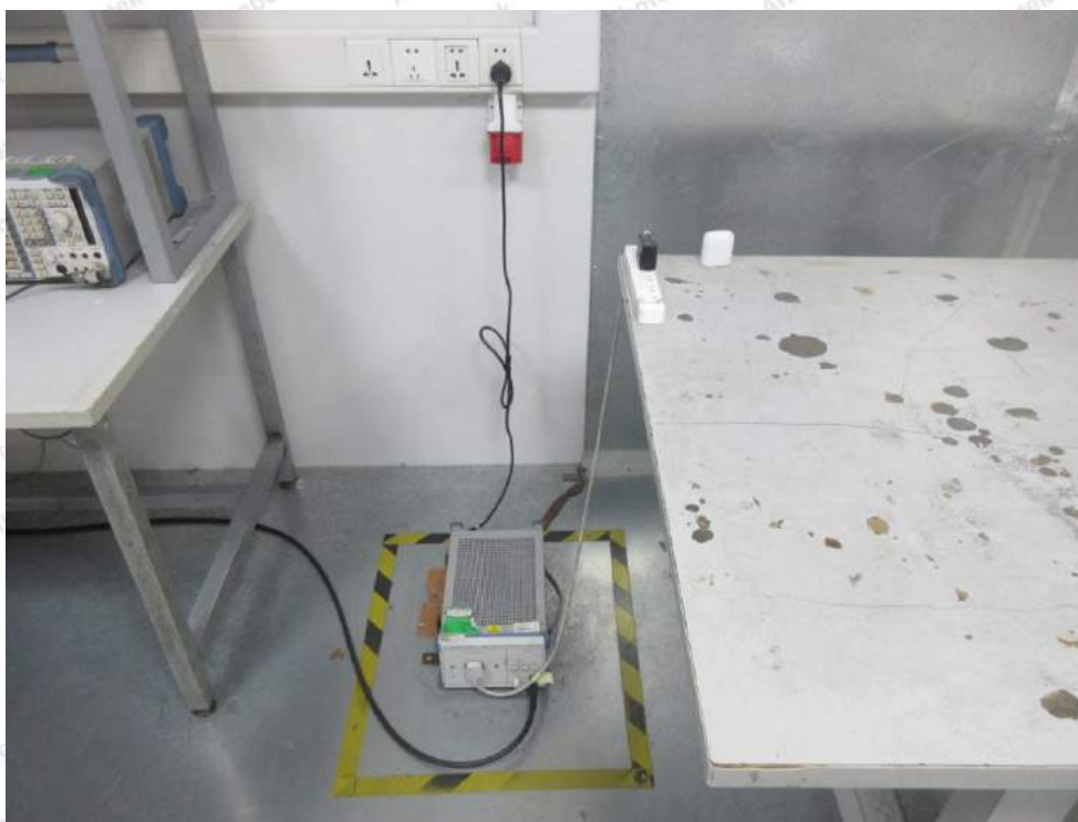
Photo of Conducted Emission Measurement
