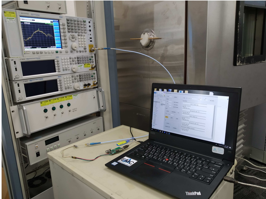
Photograph 4: Set-up for Conducted testing
