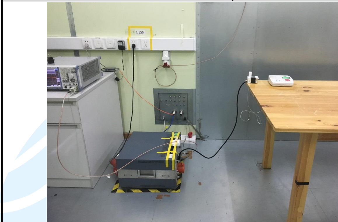
Conducted Emission Test Setup - Mode 1
