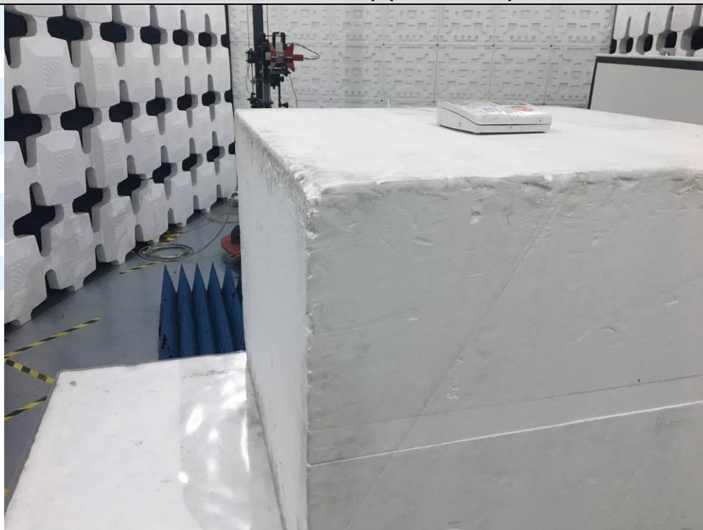
Radiated emission Test Setup (Above 1 GHz) - Mode 3
