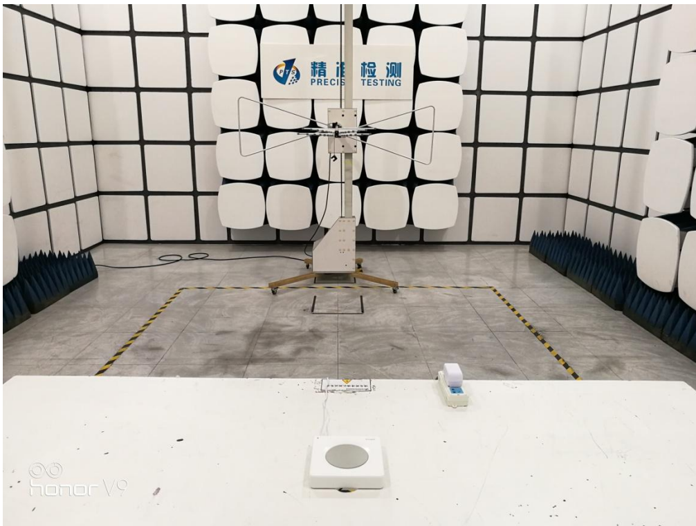
RADIATED EMISSION TEST SETUP ABOVE 1GHz
