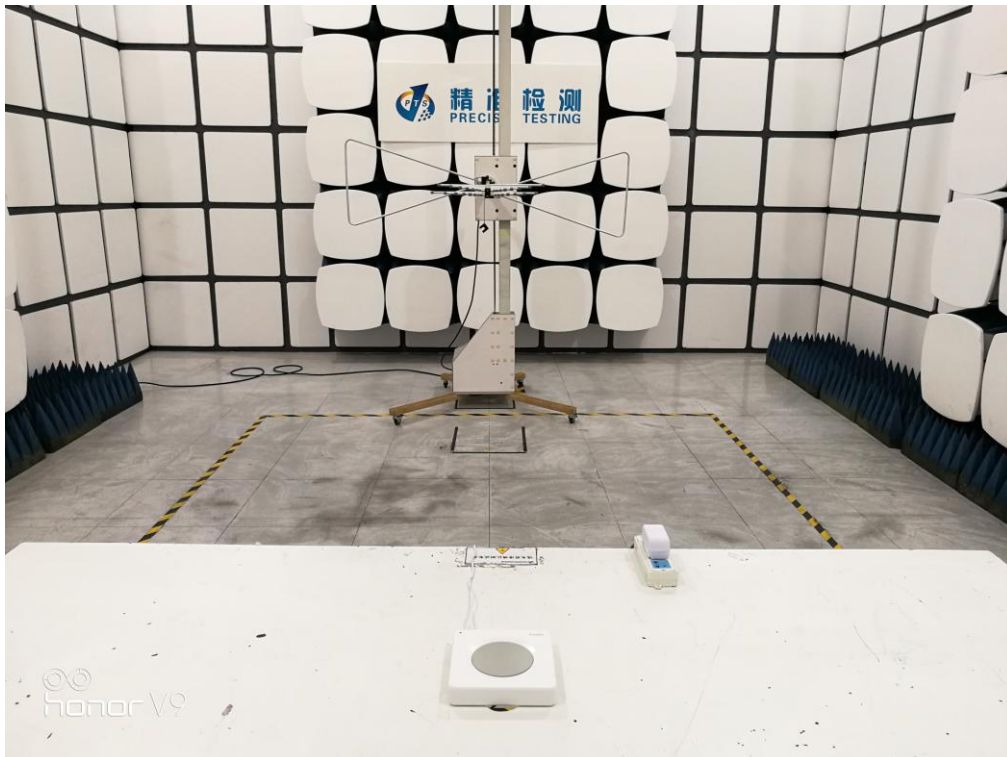
RADIATED EMISSION TEST SETUP BELOW 1GHz-CYY
