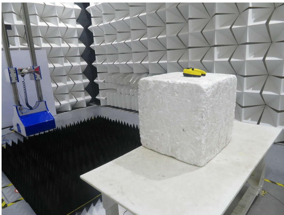
Radiated spurious emission Test Setup-3(Above 1GHz)
