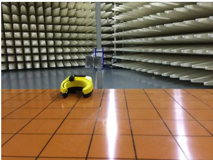
Spurious Radiated Emissions Test setup (1GHz~25GHz)
