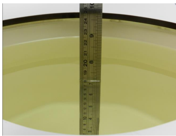
Fig 11.2 Photo of Liquid Height for Body SAR
