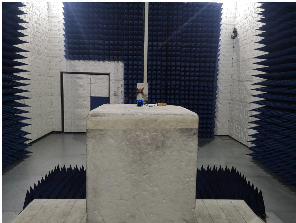
RADIATED EMISSION TEST SETUP ABOVE 1GHZ
